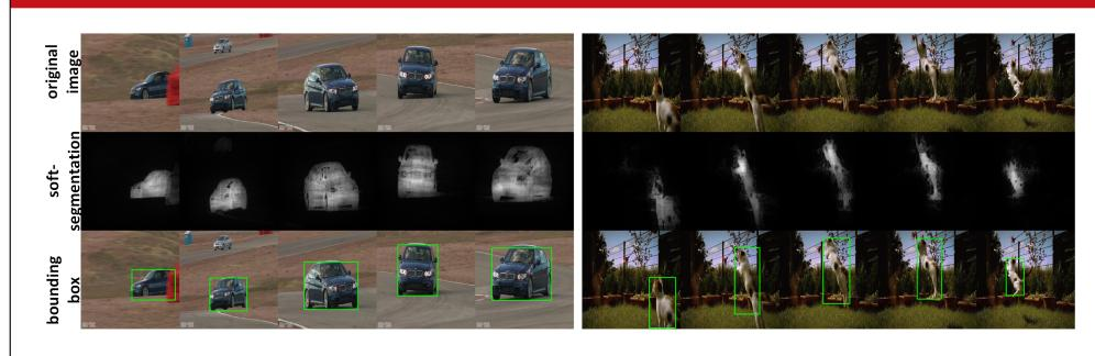
In the first example the appearance model of the car is sufficient for correct object segmentation. In the second example the motion model plays an important role in the discovery of the cat.
