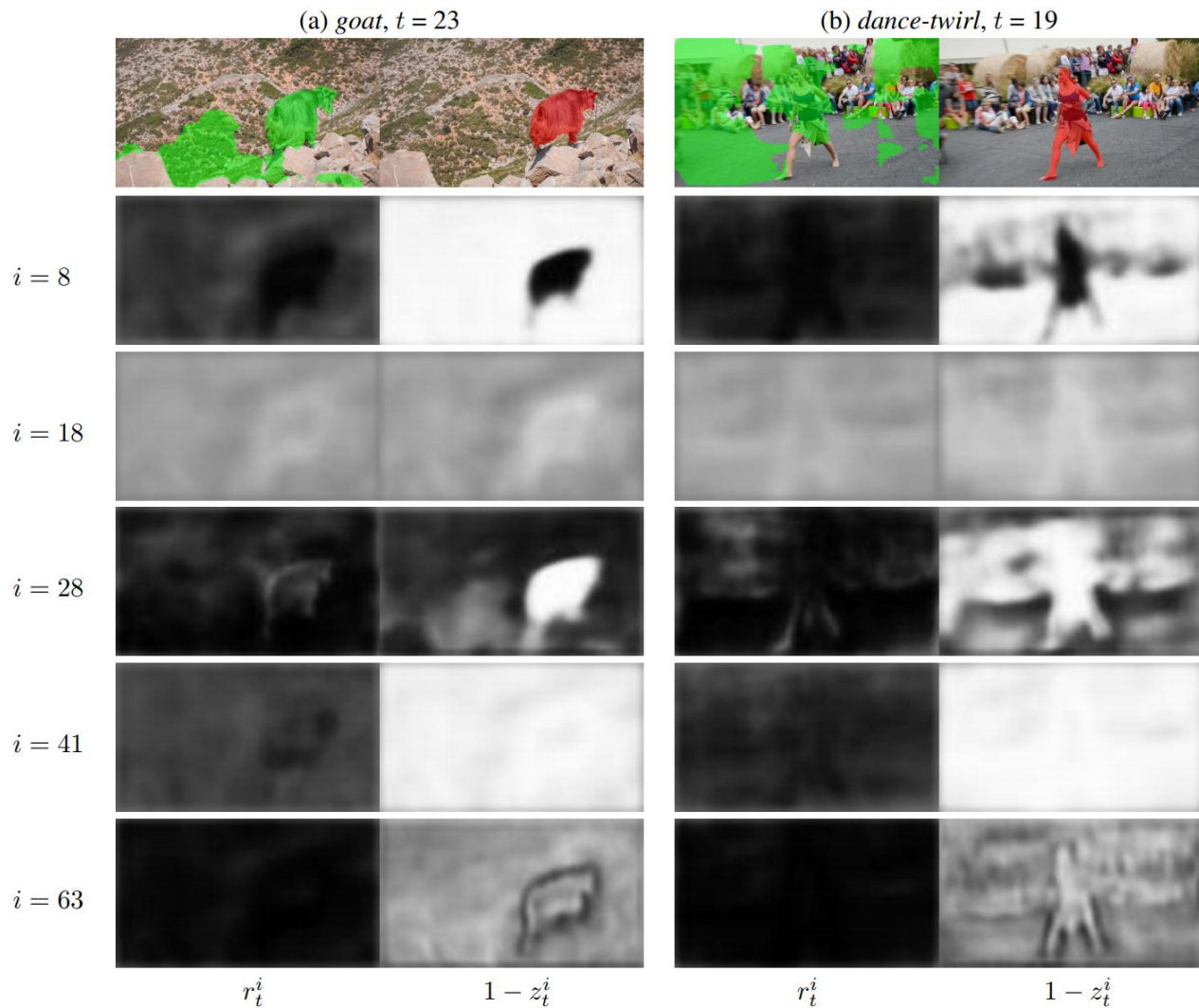
Figure 7. Visualization of the ConvGRU gate activations for two sequences from the DAVIS validation set. The first row in each example shows the motion stream output and the final segmentation result. The other rows are the reset ( r_t ) and the inverse of the update ( 1 - z_t ) gate activations for the corresponding i th dimension. These activations are shown as grayscale heat maps, where white denotes a high activation.
